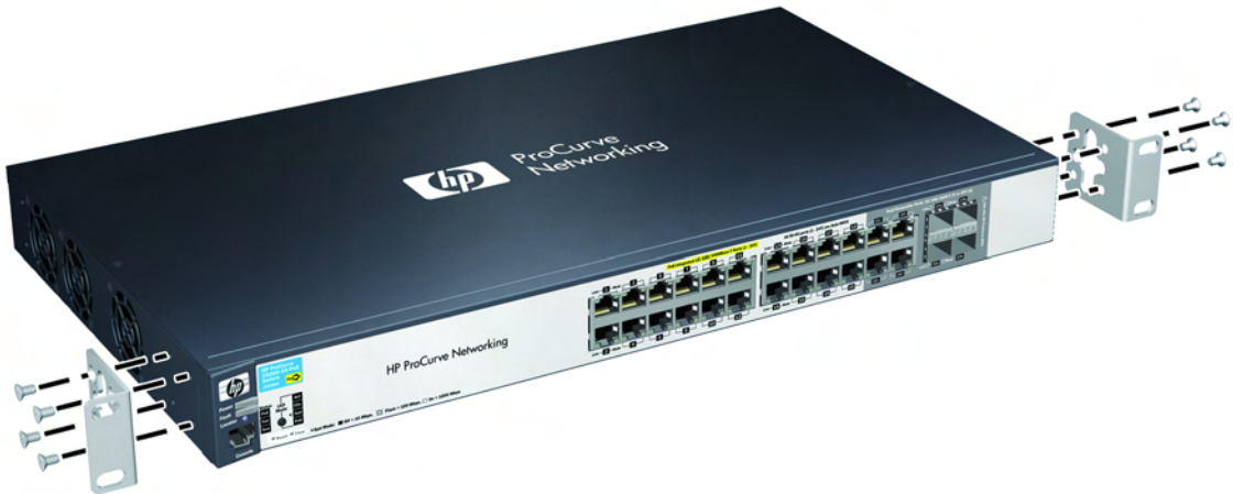
Figure 2-3. Attaching mounting brackets
